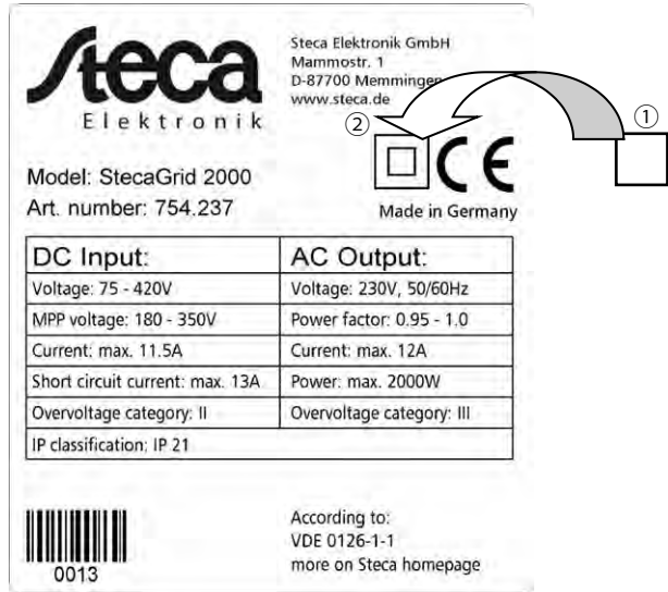
Fig. 11: Position of the sticker for covering the Protection Class II symbol
